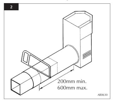
3.1.6 From outside, locate the flue assembly into the hole until the terminal is flat against the wall. Ensure the terminal is vertical. NOTE THE ORIENTATION OF THE TERMINAL. See diagram 3. Mark the four fixing holes, remove the
